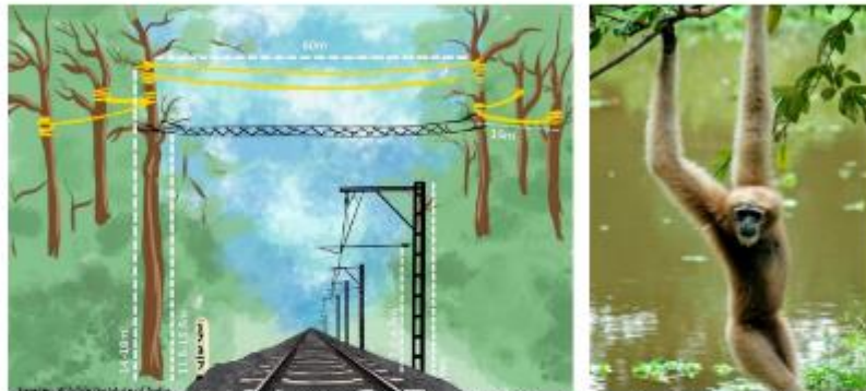
The canopy bridge designed by the Wildlife Institute of India for installation in a gibbon sanctuary in Assam, and, right, a Hoolock gibbon. SPECIAL ARRANGEMENT
