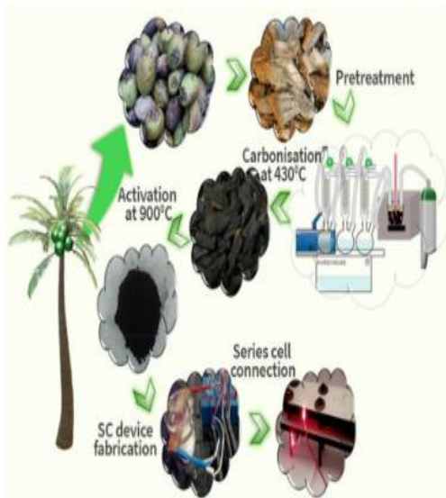
Schematic illustration of the synthesis of activated carbon.
