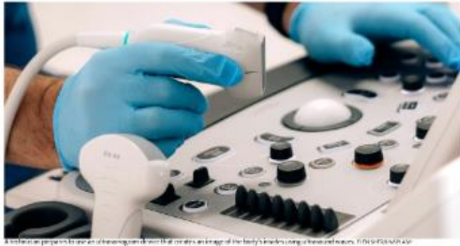
A technician prepares to use an ultrasonogram to see that certain an image of the body's tissues using sound waves. (iStockphoto.com)
